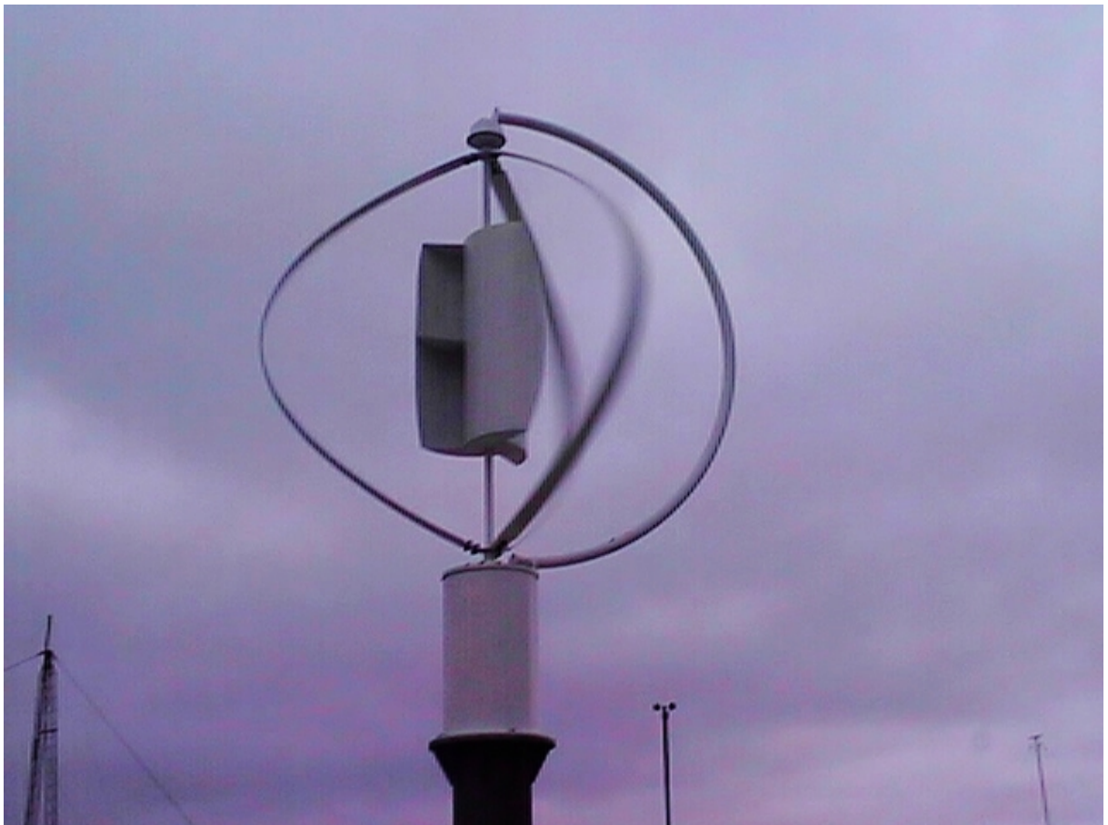
Figure 11: A Darrieus turbine (generating most of the energy), surrounding a Savonius Turbine (self-starting, to get the Darrieus moving).
