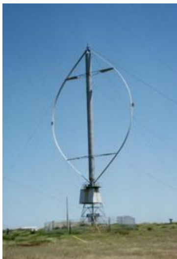
Figure 10: A Darrieus Wind Turbine
