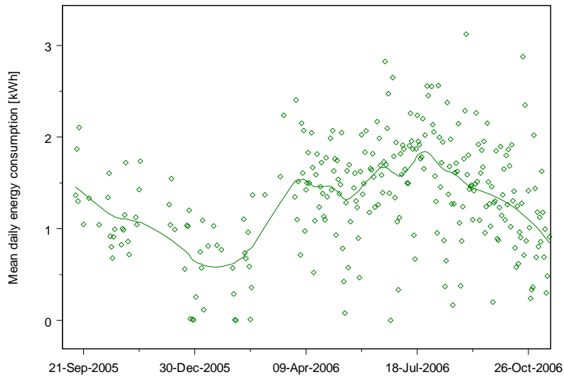
Figure 9: Daily energy use for the Waitakere NOW Home® lighting
