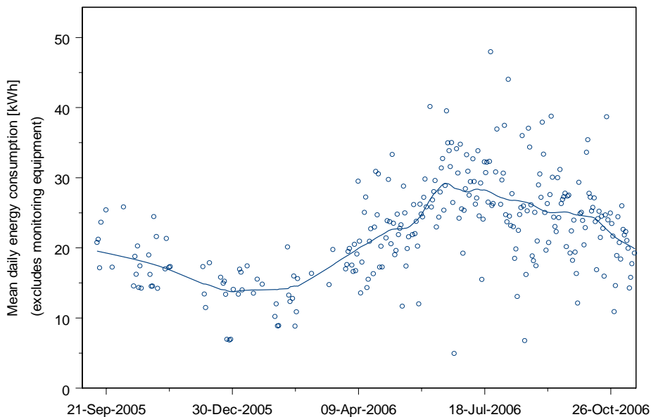
Figure 3: Mean daily purchased energy (electricity) consumption for the Waitakere NOW Home®
