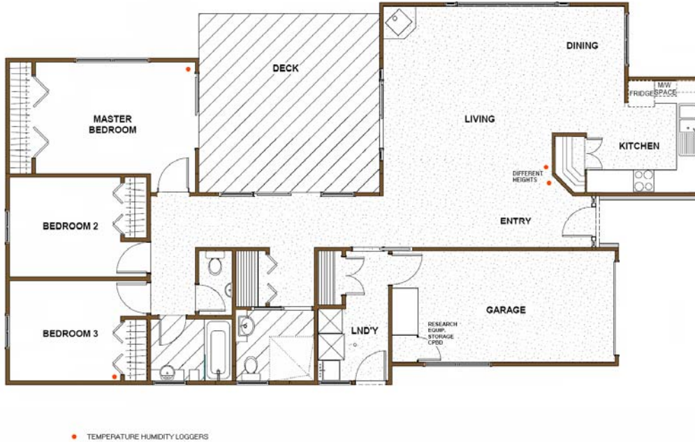
Figure 3 Floor plan of the Rotorua NOW Home® showing temperature sensor locations
