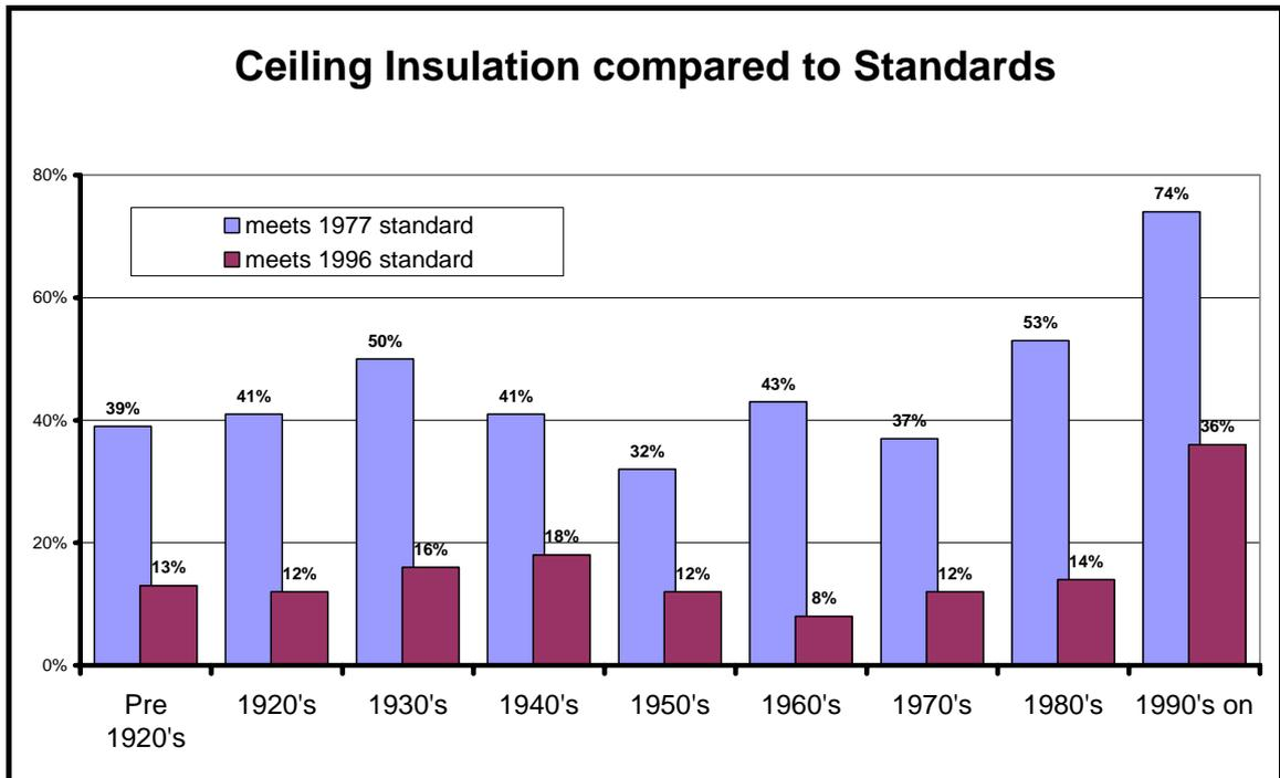
Figure 3: Ceiling insulation standards in surveyed houses. (NZHCS, 2005)
