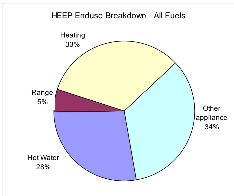
Figure 2. Breakdown of energy use in New Zealand houses. (HEEP 2006)
